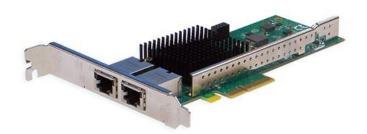
The Silicom's 10 Gigabit Ethernet PCI Express server adapters are based on Intel X550. The Intel X550 10 Gigabit Ethernet controller includes two fully integrated Ethernet Media Access Control (MAC) and two fully integrated 10GBASE-T copper PHYs.
