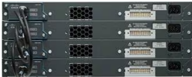
Figure 2. Cisco FlexStack Switch Stack
